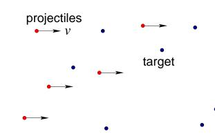
Due to interactions, targets and projectiles "see" each other as spheres of projected area  $\sigma(v)$ : the **cross section**
