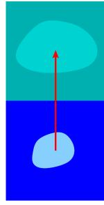
consider blob of gas in star, displaced upward expands to match lower surrounding pressure
